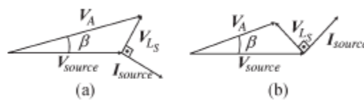
Fig. 5. Phasor diagrams. (a) Delivering active and reactive power. (b) Delivering active and absorbing reactive power.
