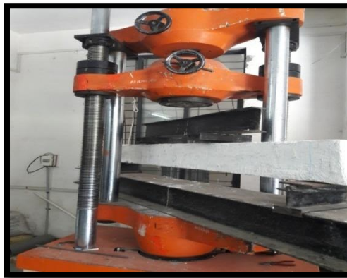
PhotoNo.6: Digital Universal Testing Machine of 100 tones capacity
