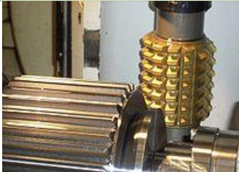
A gear hob in a hobbing machine with a finished gear.
