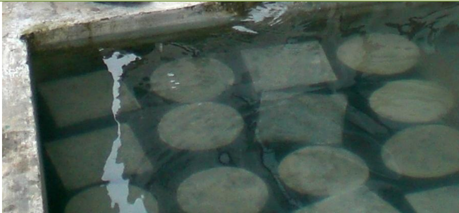
Fig 2.4 Curing of specimens in water
