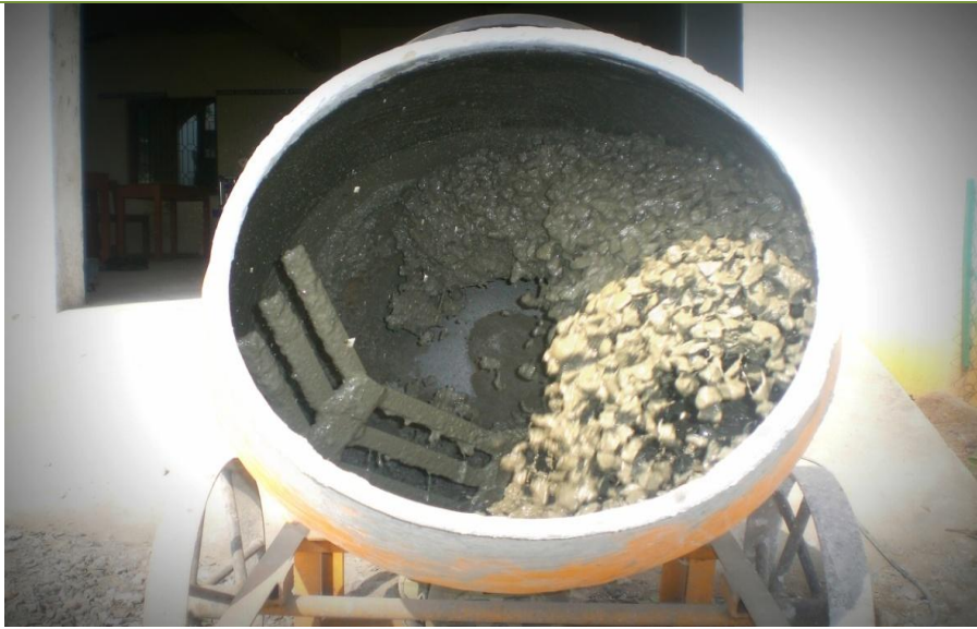
Fig 2.1 Mixing of concrete for preparing cube moulds
