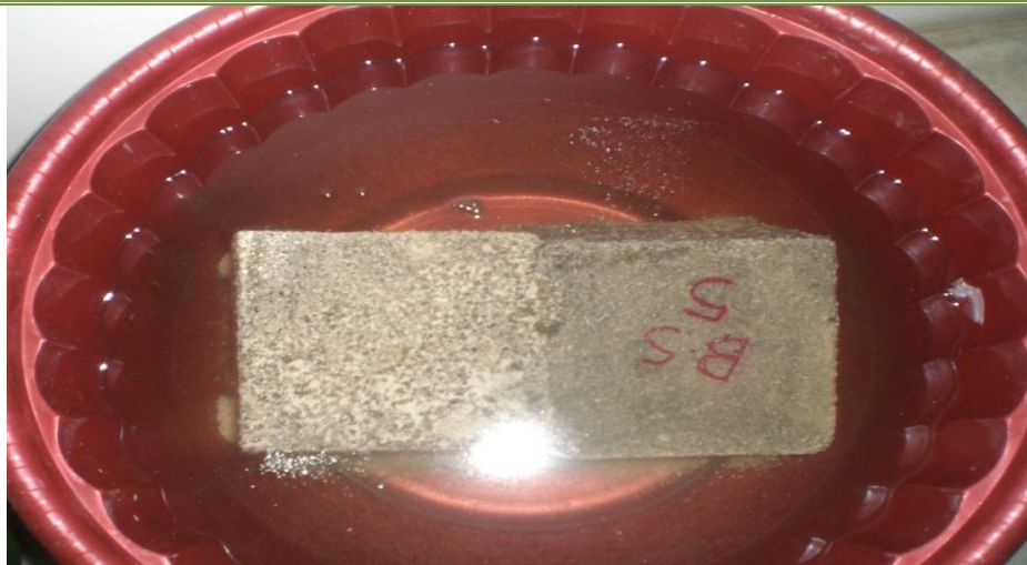
Fig 2.7 Analyzing chemical attacks on concrete specimens
