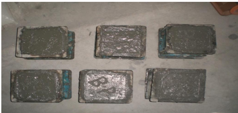
Fig 2.2 Cube moulds were made and dried for one day
