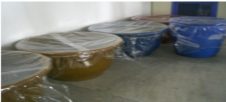
Fig 2.5 Curing of specimens in bacterial solution
