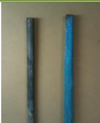
Fig 1.6 FRP coated rebars
