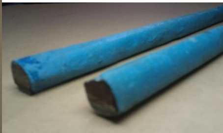
Fig 1.7 Side view of coated rebar
