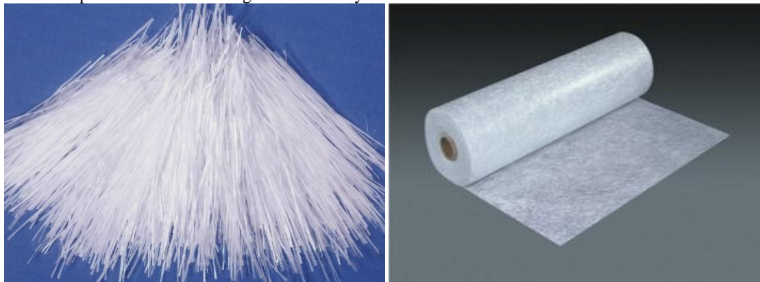
Fig 1.4 E-glass chopped strands Fig 1.5 E-glass chopped strand mat
