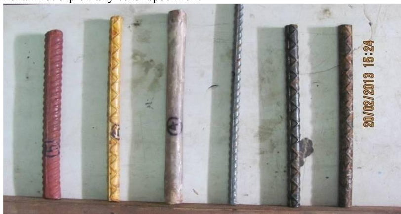
Fig 5.5 Specimens for salt spray test
