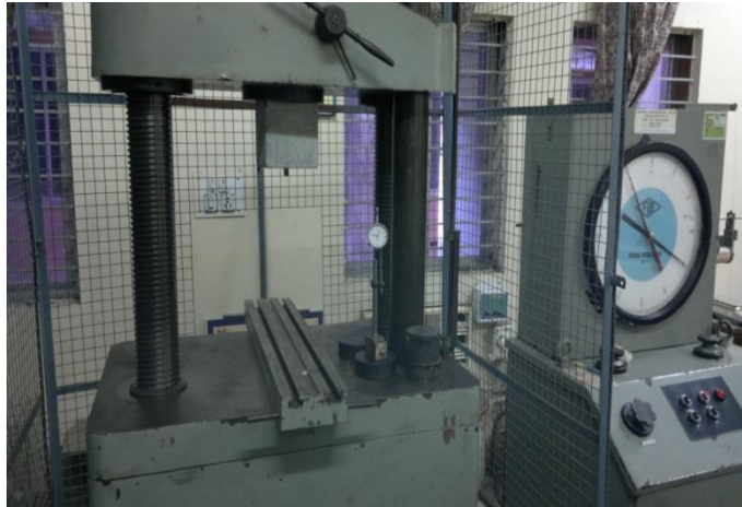
Fig 5.10 Secure the sample in UTM
