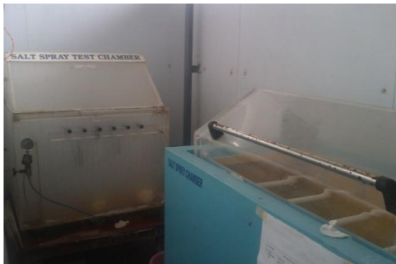
Fig 5.6 Saltspraychamber Fig 5.7Placingthe rebar
