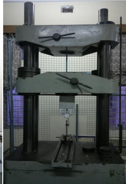
Fig 5.11 Pull-out loading setup
