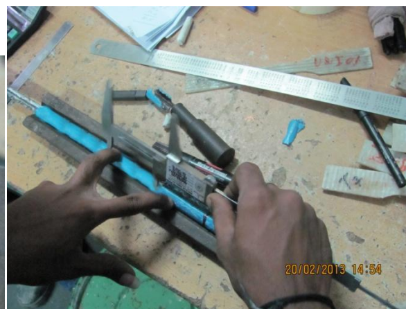
Fig 5.2 Marking gauge length
