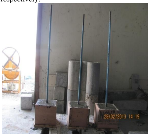
Fig 5.8Rebar setup in mould
