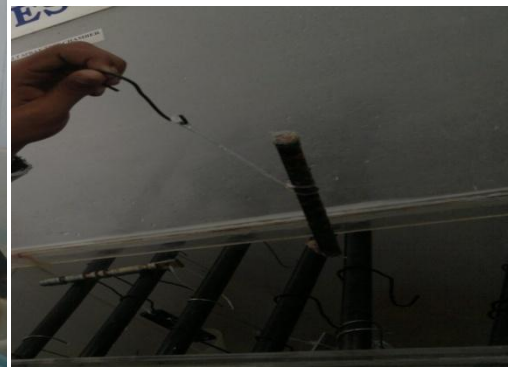
Fig 5.6 Saltspraychamber Fig 5.7Placingthe rebar
