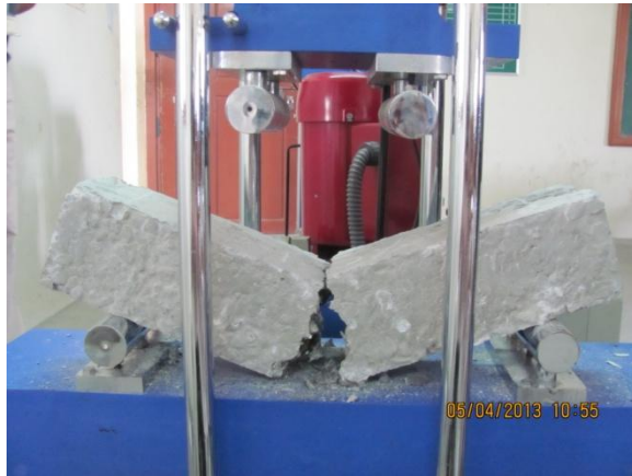
Fig 5.14 Failure of beam
