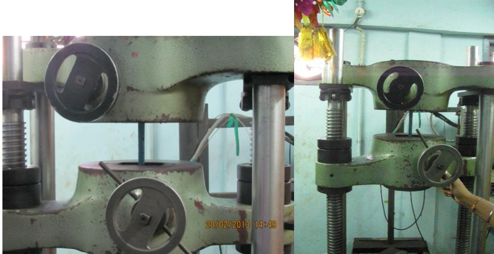
Fig 5.3 Fix the bar in the grips of UTM Fig 5.4 Load application of UTM
