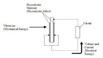
Fig1.schematic of a piezoelectric damper.
