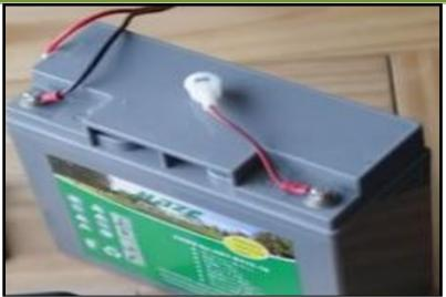
Fig. 5 lead acid battery
