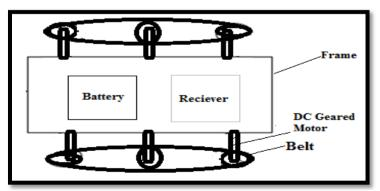
Fig. 1 block diagram of stairs climbing wheel Chair
