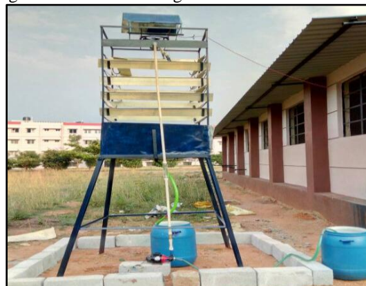
Fig. 11 assembly of cooling tower
