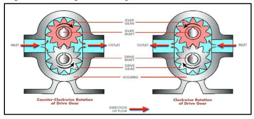
Fig. 4 working of pump
