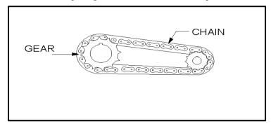
Fig. 3chain drive with sprocket
