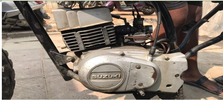
Fig. 3.5 Two-Stroke Petrol Engine
