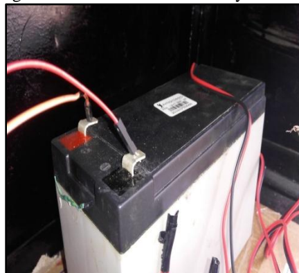
Fig. 5 lead acid battery
