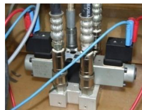
Figure 1; A hydraulic servo valve; Figure 2; Photo of high performance hydraulic servo valve
