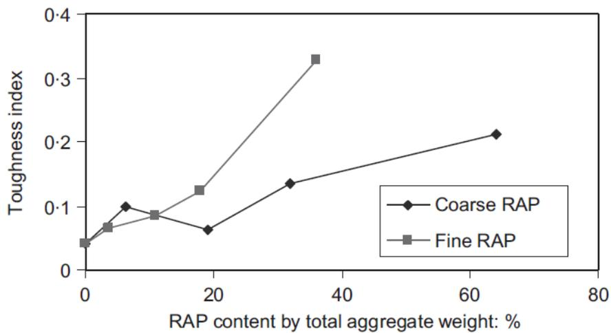
**Fig. 3** Relation between Toughness index and RAP content. [5]
