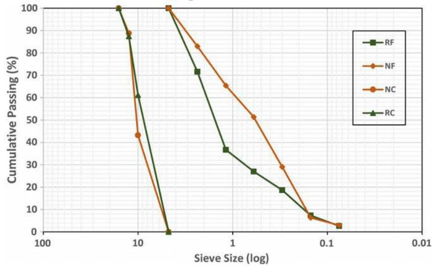
**Fig.1** Grain size analysis of natural and RAP aggregates [31]
