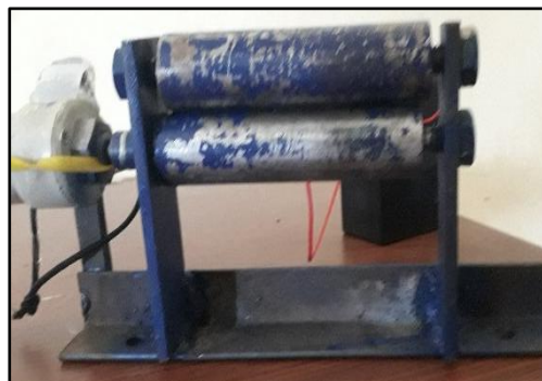
Fig. 8 Rollers with Supporting Frame
