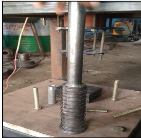
Fig. 4 Plunger with Spring
