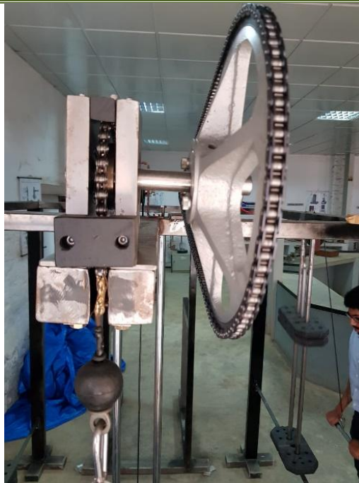
Figure 5.2: Shaft connecting geared pulley and pinion
