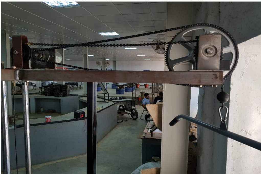
Figure 5.1: Pinion gear and dynamo gear coupled by chain drive
