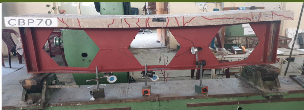
Figure 13: Cracks pattern and mode of failure for CBP70 specimen
