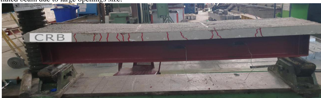
Figure 9: Cracks pattern and mode of failure for CRB specimen
