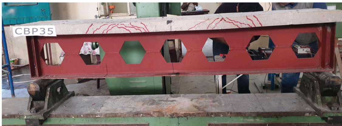
Figure 11: Cracks pattern and mode of failure for CBP35 specimen
