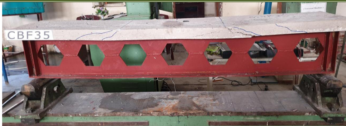
Figure 10: Cracks pattern and mode of failure for CBF35specimen
