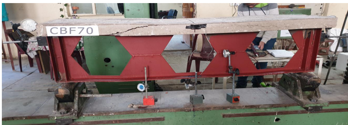
Figure 12: Cracks pattern and mode of failure for CBF70 specimen
