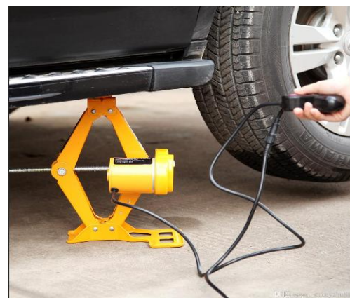
Fig. 3 working of motorized jack
