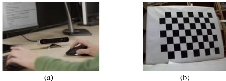
Fig. 1 Camera calibration setup (a), and image pattern for calibrating intrinsic parameter (b)
