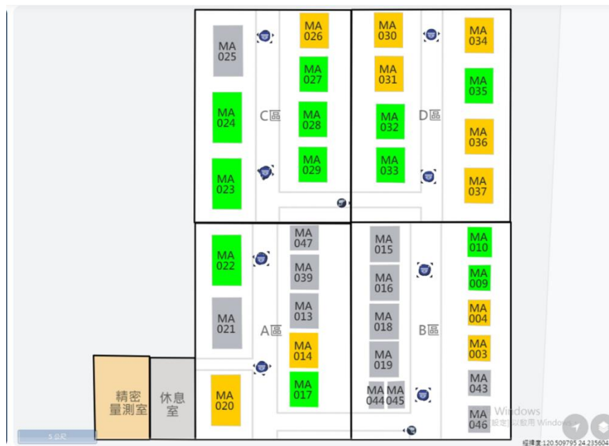
Figure 13. Real-time Status of Operational Analysis for Each Machine (Dashboard)
