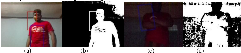
Fig.2:Low light environment ((a)-original with HOG and CamShift, (b)-mask image with HOG), High light environment ((c)-original with HOG and CamShift, (d)-mask image)
