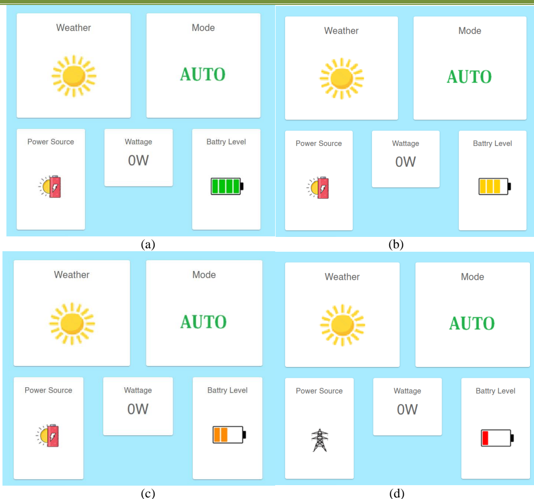
Figure 11: IoT web interface is updated according to voltage level of the battery
