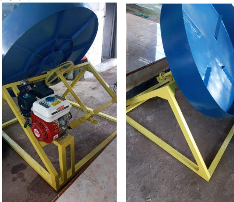
Figure 1 Designed organic fertilizer granulation machine (pan granulator).
