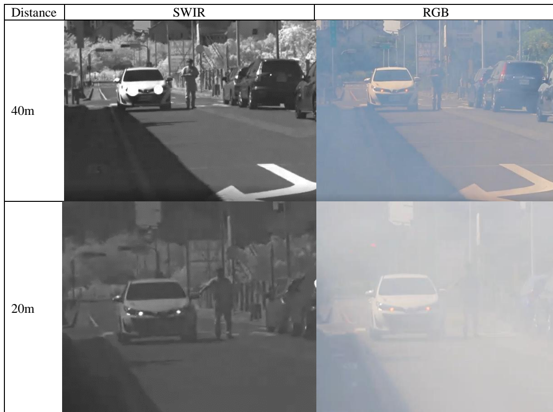
Fig. 10 Tested in smoke at different distances.
