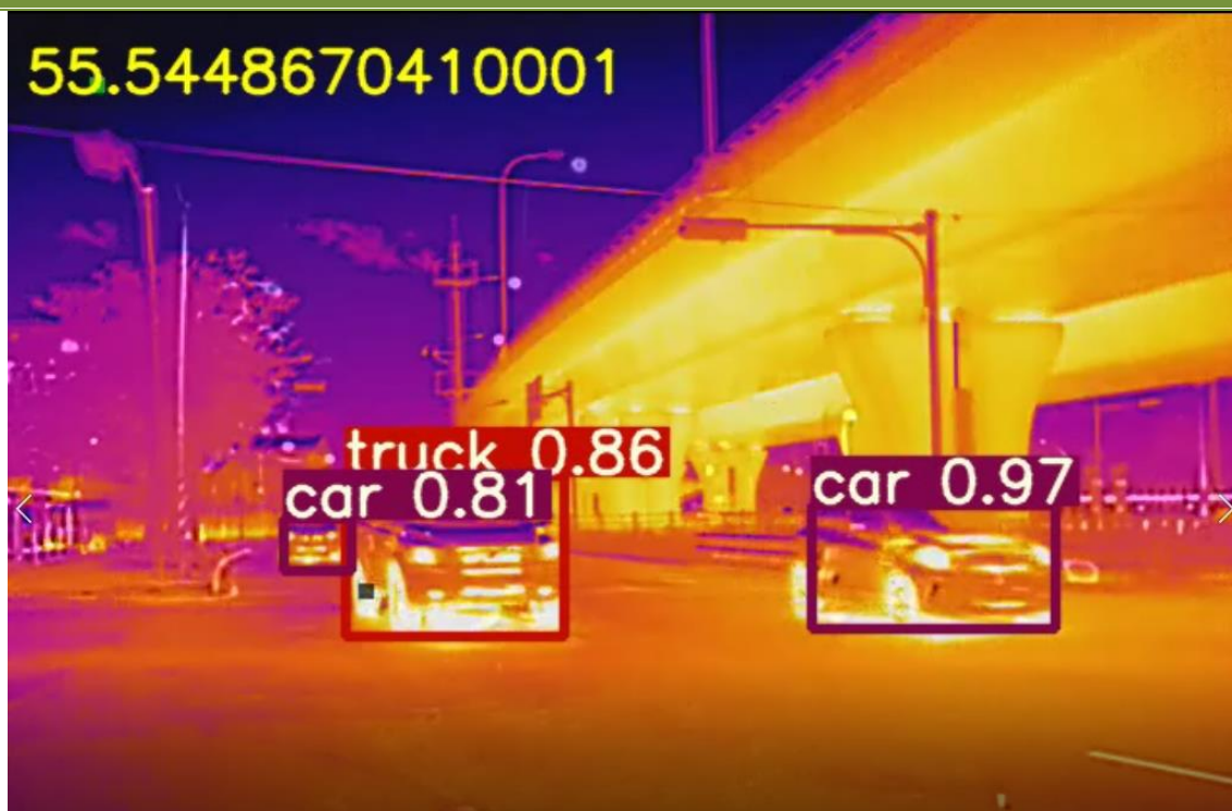
Fig. 14 Thermal imaging mistakenly identified regular cars as trucks
