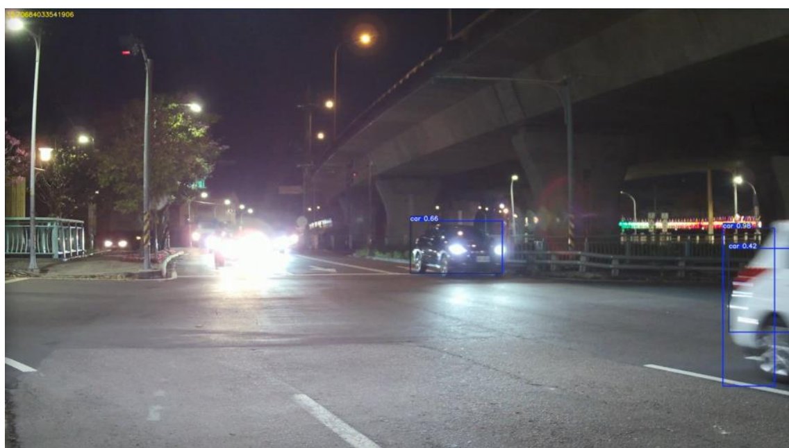
Fig. 17 Recognition results of optical images under the influence of car headlights
