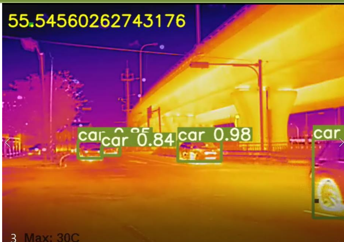
Fig. 18 Recognition results of thermal imaging under the influence of vehicle headlights
