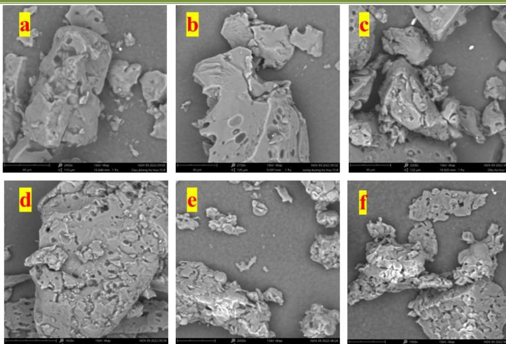
Figure 5. SEM images of hydrogenated RS5 samples: Peanut (a), sunflower (b), olive (c), soybean (d), stearic acid (e), palmitic acid (f)
