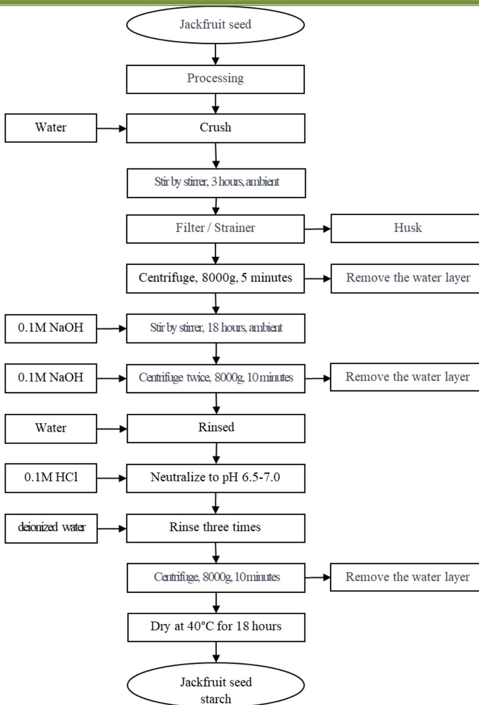
Figure 1. Process Flowchart for Extracting Jackfruit Seed Starch
