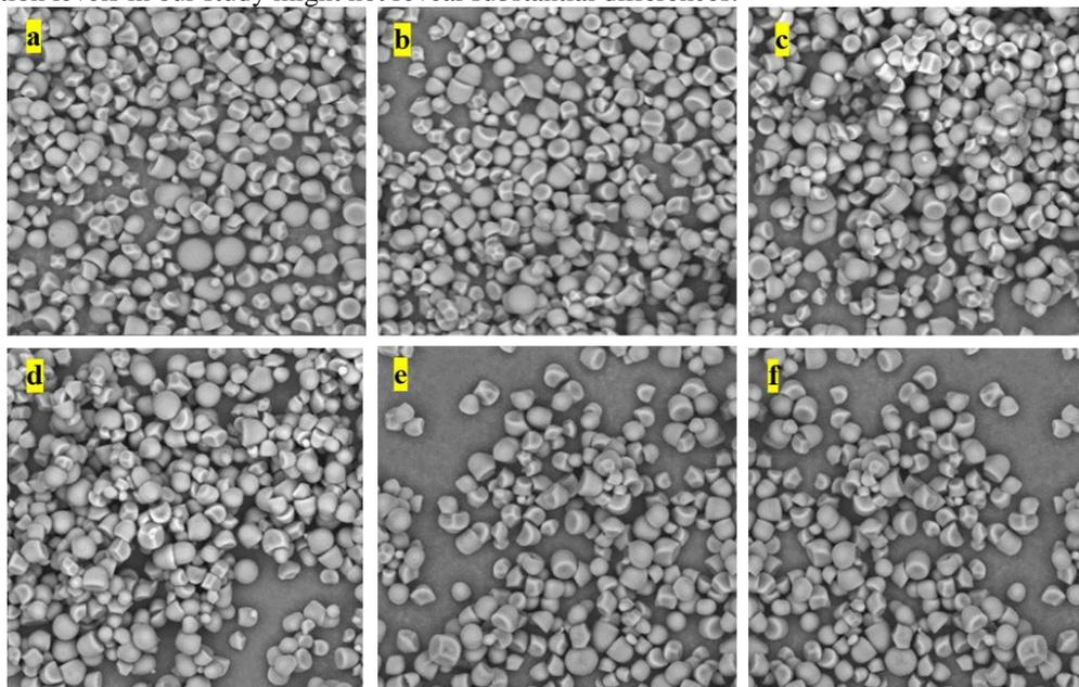
Figure 4. SEM images of non-hydrogenated RS5 samples: peanut oil (a), sunflower oil (b), soybean oil (c), olive oil (d), stearic acid (e), palmitic acid (f)
