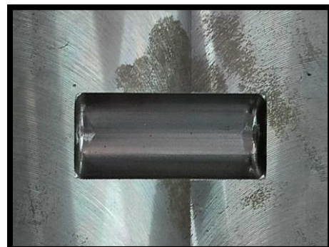
Fig: 6 Hardness Specimen Mould According to ASTM E-10 Standards.
